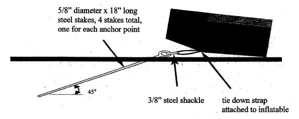
If the unit is on cement or any hard surface, to protect the base or the unit from abrasion, make sure that you have put a tarp down and placed the unit on it before inflating it. Use sand bag pouches that can carry a minimum of 100 lbs tension load per anchor point. Connect the tie down straps to the sand bag pouches. Remember to install sand bags at such distance from the ride that the ride straps connected to the shackle would be taut.
