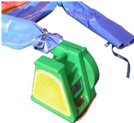
6. Twist the vent (the other tube) several times, fold it over and secure snugly with the attached strap.
